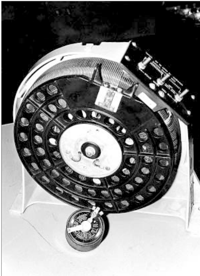
Figure 4.2. This photo shows the working parts of two autotransformer dimmers, 6 kW and 100 Watts. The 6 kW unit was commonly installed as a replacement for resistance dimmers and was made to fit into the same space. The 100 watt unit served as a master controller for ranks of resistance-based individual circuit controllers in early preset consoles.
